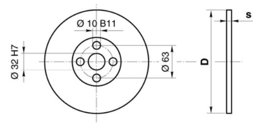
Best performance of crownscrew is guaranteed when circular saw blades with drawing holes are used
